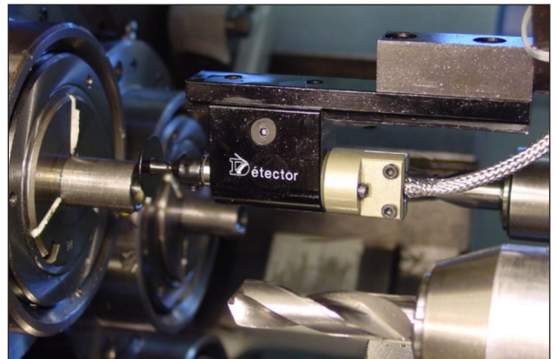
A Solartron Probe is mounted into this Detector Length Measurer
