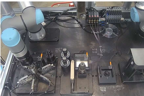
Air Gauging (Center) with AGM connection on top. Photo courtesy of Arnold Gauge (West Chester County, OH, USA)
