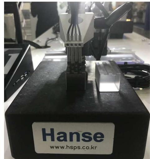
3mm probes checking different ridges.
