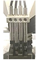
3mm probes checking ridges
