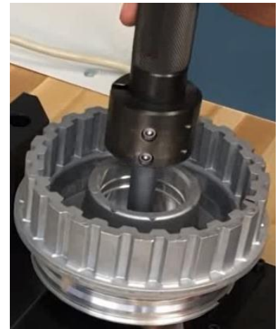
DZ Probes being used to check runout. Photo courtesy of VGage Gauging Systems ( www.vgage.com )
